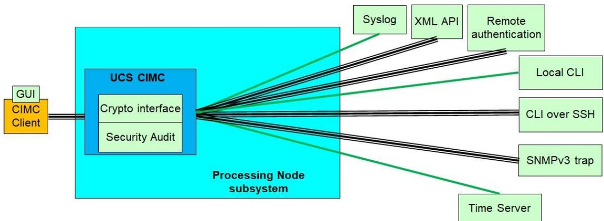
Figure 1: TOE Architecture
