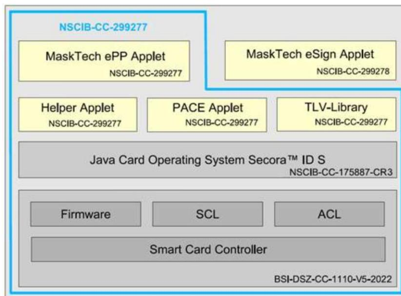
The light yellow blocks represent the applets provided by the developer that together yield the MaskTech ePP Applet on Secura™ ID S v1.1. Only the components surrounded by the blue outline are part of TOE.
